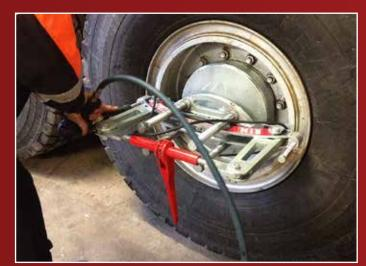
Put the new o-ring around Rim Wizard before you tighten the bolts so that it is easy to install. Then tighten the two bolts which will push the lock ring forward.
