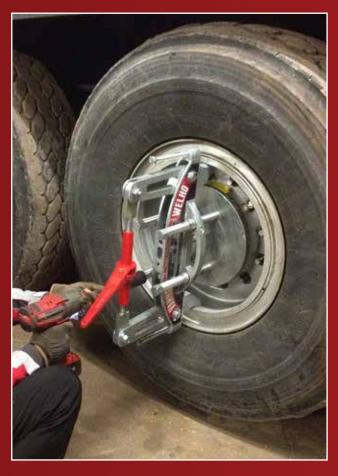
Tighten the four bolts in Rim Wizard alternately as long as the rim comes out from the hub.
