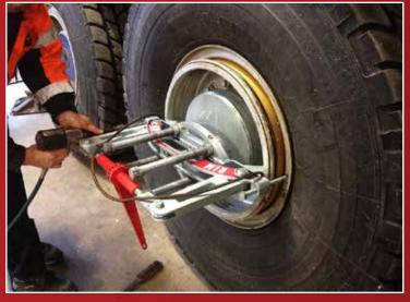
When o-ring is set, loosen the bolts in Rim Wizard. Start filling the tire.
