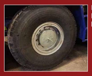
Lift the wheel into the air. Put the hub cover on and tighten it with the bolt in it. Let the air out of the tire.
