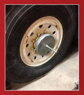
Put the hub cover on and tighten it with the bolt in it.
